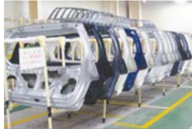
22. RACK FOR PAINTED BACK DOOR
