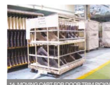
14. MOVING CART FOR DOOR TRIM PICKNG
