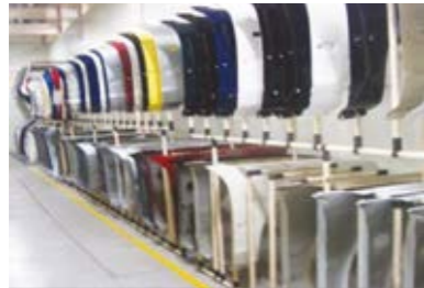
16. RACK FOR PAINTED PARTS
